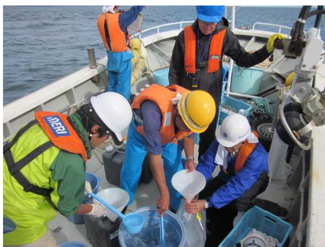
海水の採取後、均一化した後、原子力規制庁の容器と I A E A の容器に分別。 これらの試料は日本、I A E A モナコ海洋環境研究所にて分析予定。 Distribution of seawater samples to NRA containers (left) and IAEA containers (right) after collection and homogenisation. The samples will subsequently be analysed in parallel in Japan and the IAEA Environment Laboratories in Monaco.
