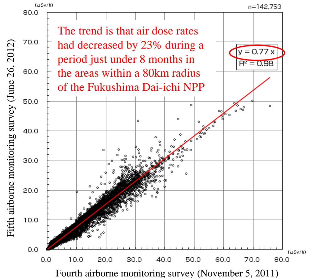
Figure: Relationship between the results of the fourth airborne monitoring survey (air dose rates) and those of the fifth airborne monitoring survey (air dose rates)
